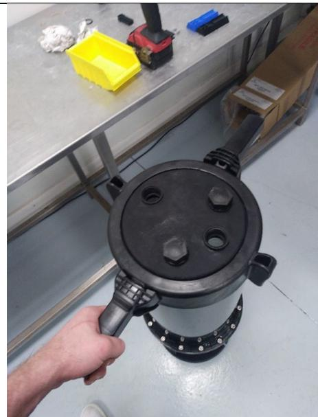
8. Then use the handles to **finish tightening about fifteen centimeters**
