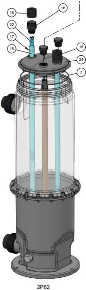
Figure 1: Exploded zoom reactor
