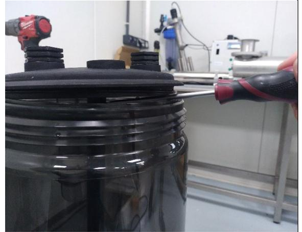
6. Help insert the connecting tube into the middle part of the lid (using a fine tool, flat screwdriver, strip, etc.)
