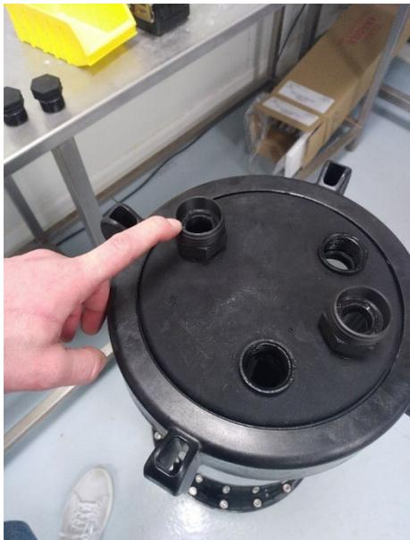
11. Install seals and **tighten by hand.** It's over.
